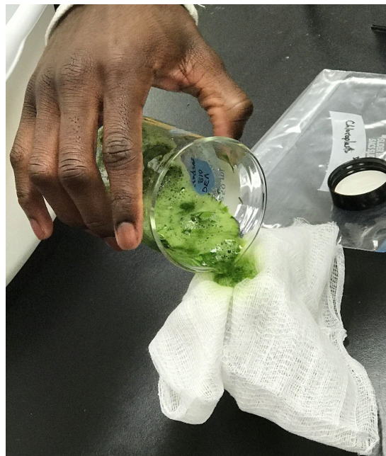
Figure 3: In this picture you can see Fon separating solid from liquid. We only need the liquid when using the centrifuge.
